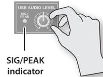
To check the volume level of the USB audio being output, you can use the level meter displayed on the USB Streaming screen or the SIG/PEAK indicator on the top panel.
